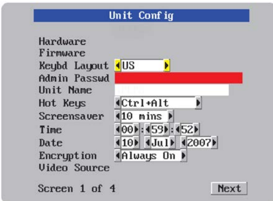
Figure 6. Unit Configuration OSD
