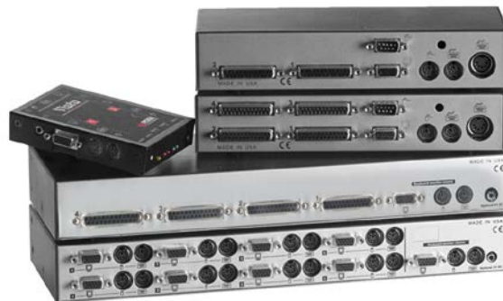
Rear view of Vista models KVL-8PCA, KVL4UA, KVT-2PC, KVM-4UPH, KVM-2UPH
